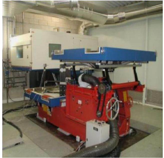
Fig. 1. The vibrating platform.
